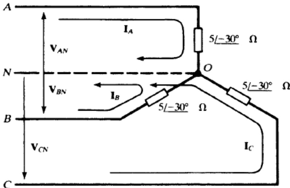
$$\begin{aligned} \vec{U}_{AB} &= 150 \angle -120^\circ \\ \vec{U}_{BC} &= 150 \angle 0^\circ \\ \vec{U}_{CA} &= 150 \angle 120^\circ \\ \vec{U}_{AN} &= \frac{150}{\sqrt{3}} \angle -90^\circ \\ \vec{U}_{BN} &= \frac{150}{\sqrt{3}} \angle 30^\circ \\ \vec{U}_{CN} &= \frac{150}{\sqrt{3}} \angle 150^\circ \end{aligned}$$
