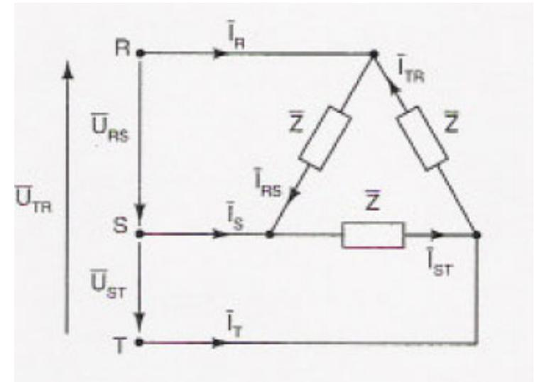
$$\vec{I}_R = \vec{I}_{RS} - \vec{I}_{TR} = I_{RS} \angle 0^\circ - I_{RS} \angle 120^\circ = I_{RS} \cdot \left( 1 + 0,5 - j \frac{\sqrt{3}}{2} \right) = I_{RS} \cdot \sqrt{3} \angle -30^\circ$$
